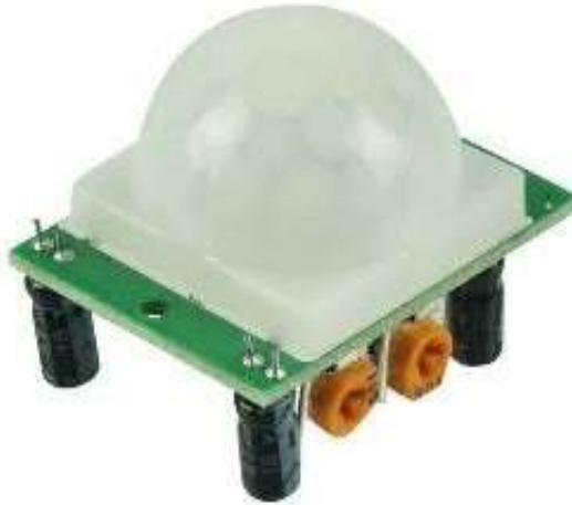
Gambar 4 Sensor PIR (Passive Infra Red)
