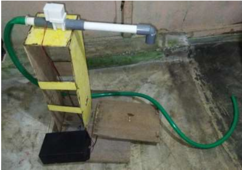
Gambar 5 Tampilan Prototype Sistem Pengisian Air Galon Otomatis Berbasis Arduino
